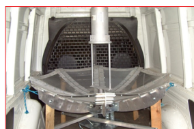
Parabolic dish antenna prototype
