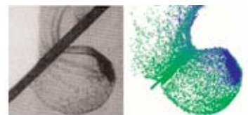
Oblique hypervelocity impact test (left) compared to analysis (right). Courtesy of UDRIS NASA.
